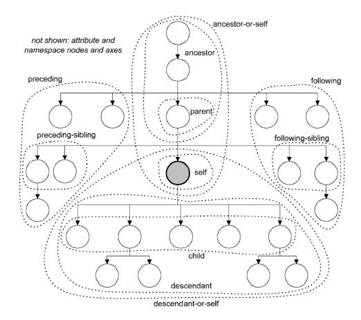
Figure 2.2: XPath axes
